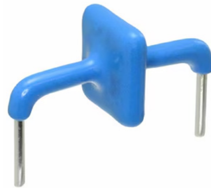
Figure 10: The AK6E-066C high-power 120 V TVS diode offers up to 10,000 A protection and is housed in a through-hole axial-lead package. (Image source: Eaton)
