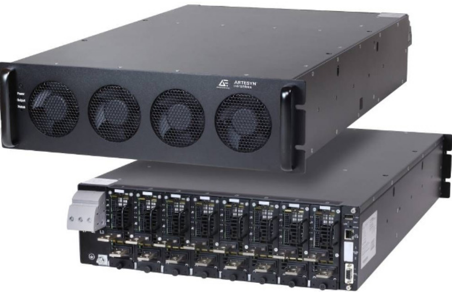
Figure 4: Advanced Energy iHP Air-Cooled Series accepts 3000 W single slot modules for up to eight different outputs for a total output power of 24 kW. (Image source: Advanced Energy)
