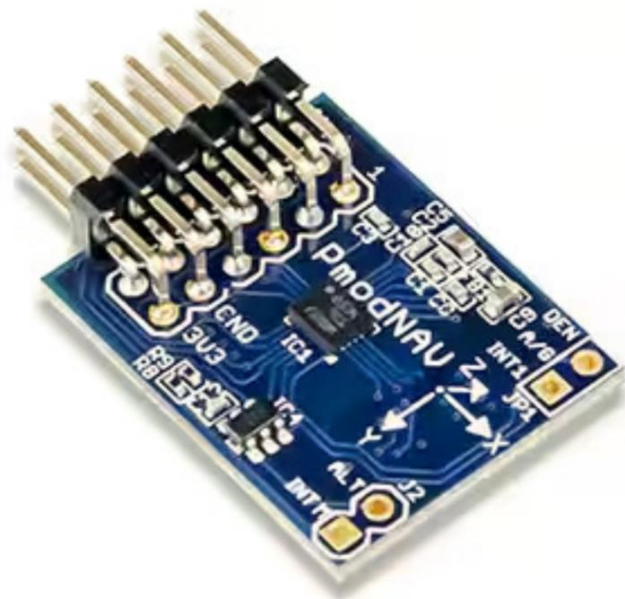
Figure 3: Digilent's 410-326 9-axis IMU/barometer uses an STMicroelectronics' LSM9DS1 iNEMU IMU that combines a 3D accelerometer, a 3D gyroscope, and a 3D magnetometer into one package. (Image source: Digilent)
