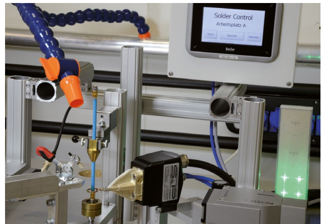
Temperature controlled soldering
